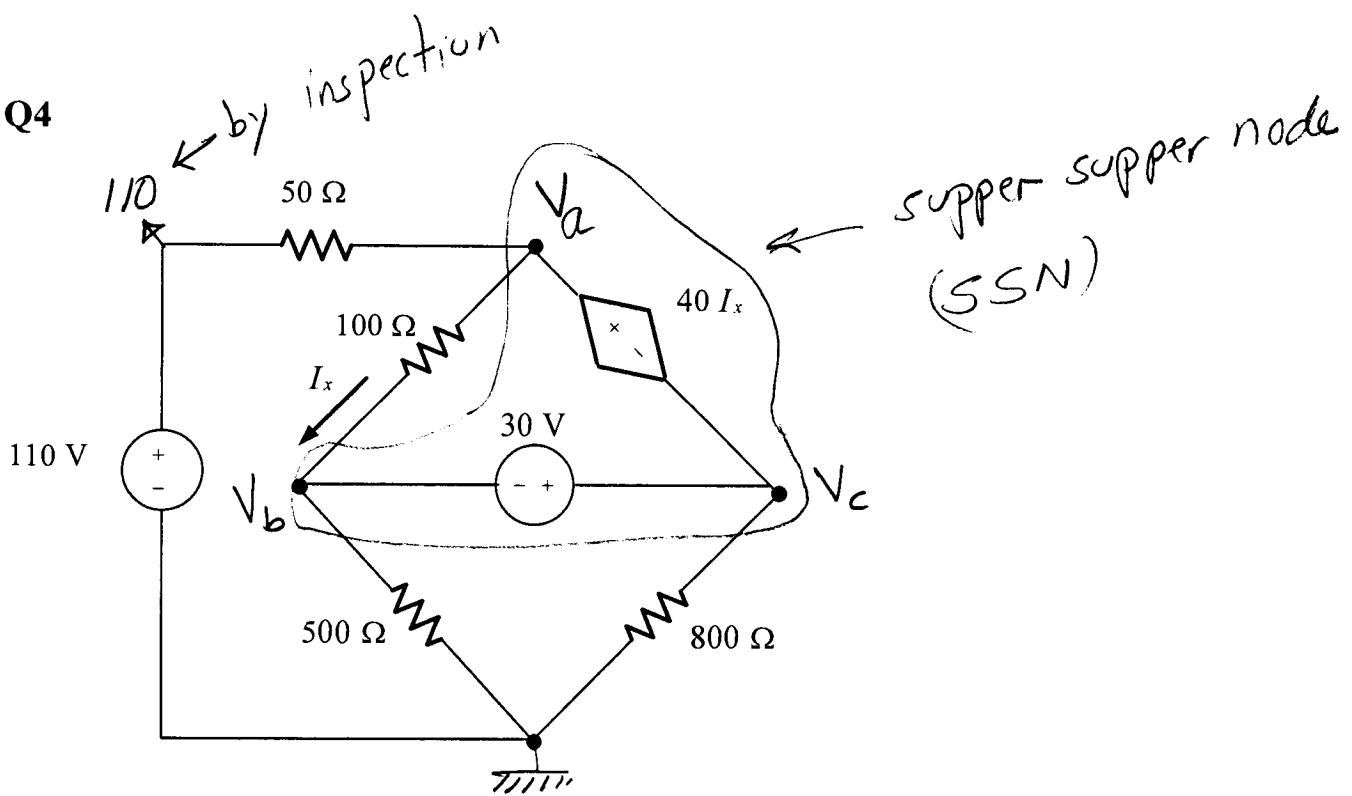
For the circuit shown above , **using the node voltage method** find the followings :
