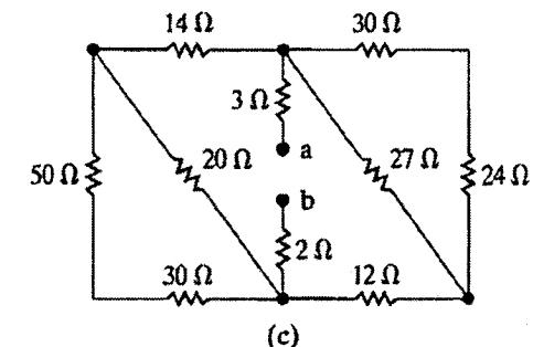
**Q1** For the circuits shown above , find the equivalent resistant between nodes a and b
