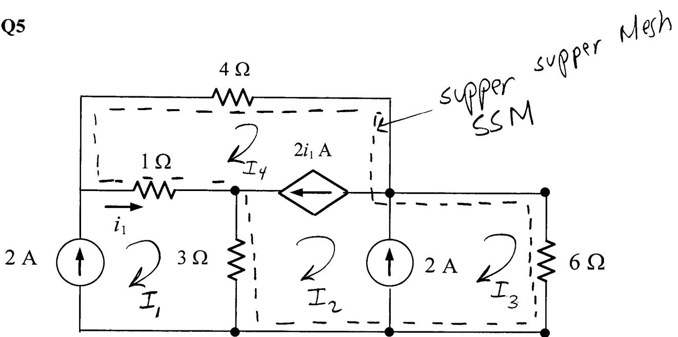
For the circuit shown above, using the **Mesh current method** find the followings :
