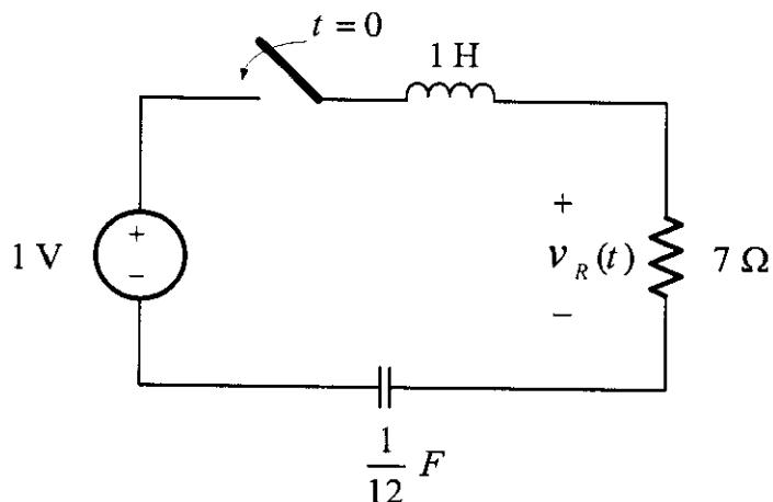
Assuming that the inductor and the capacitor has zeros initial conditions. Using the Laplace transform method , find the voltage across the resistor  $v_R(t)$
