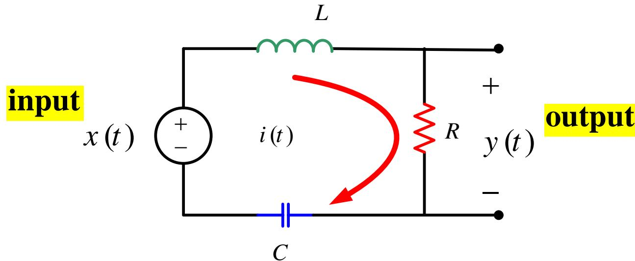
We want a relation (an equation) between the input  $x(t)$  and output  $y(t)$
