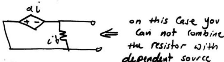
Solution: Apply a test voltage or current method
