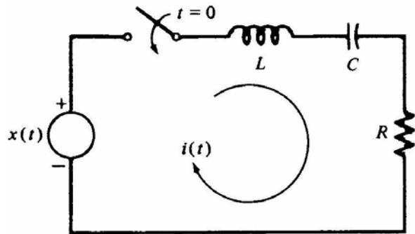
In analyzing the circuit, we first wrote down the differential equation using KVL
