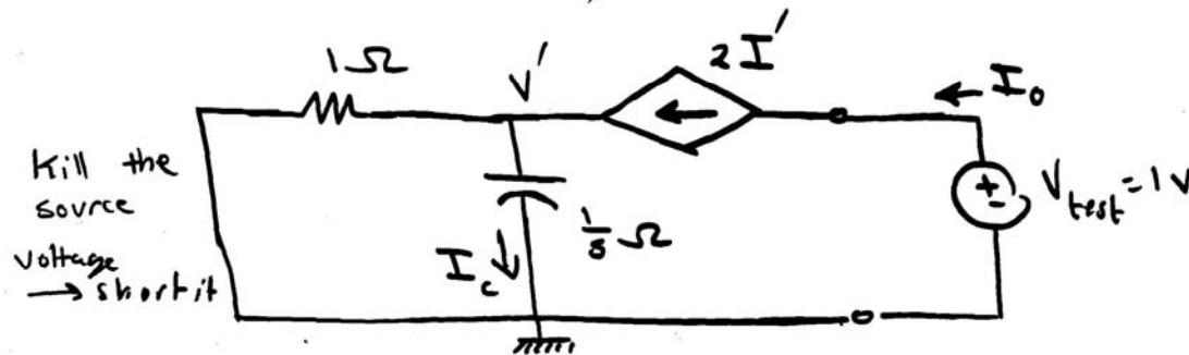
$$Z_{eq} = \frac{V_{test}}{I_o} = \frac{1}{I_o} \Rightarrow \text{Find } I_o$$
