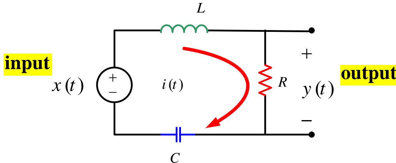
$$\underbrace{\{RC\} \frac{dx(t)}{dt}}_{\text{Term 1}} = \underbrace{\{LC\} \frac{dy^2(t)}{dt^2}}_{\text{Term 2}} + \underbrace{\{RC\} \frac{dy(t)}{dt}}_{\text{Term 3}} + \underbrace{\{1\}y(t)}_{\text{Term 4}}$$
