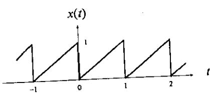
$$T_0 = 1 \Rightarrow f_0 = 1 \text{ Hz}$$
