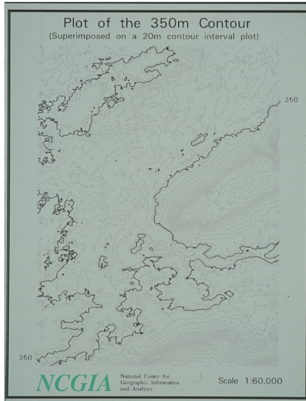
Plot of the 350 m contour for the State College, Pennsylvania, U.S.A. topographic quadrangle. The contour has been computed from the U.S. Geological Survey's digital elevation model for this area.
