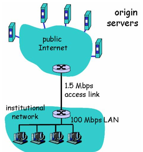
Overall delay= few seconds + minutes + few milliseconds  $\approx$  few minutes which is very large and the network designer must avoid such delay.
