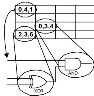
Fig. 2. Example of a circuit and its encoding
