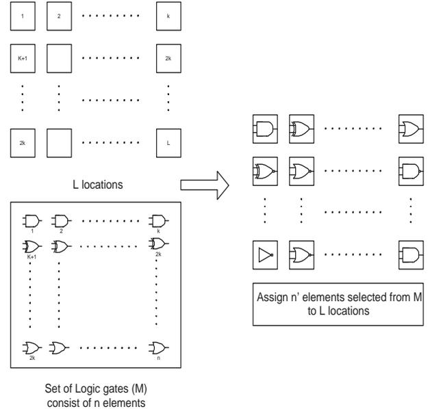
**Fig. 6.** Representation of digital logic design problem.
