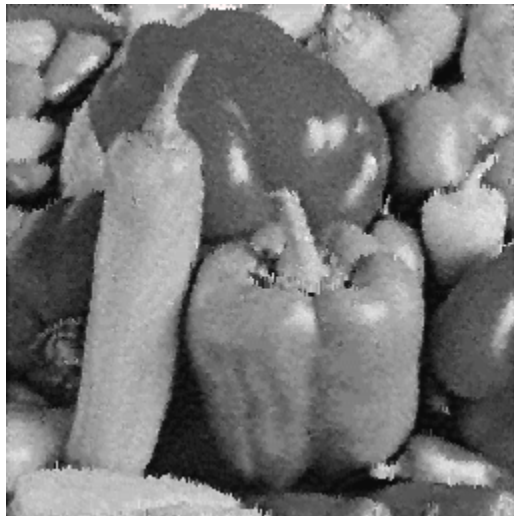
Figure 9. Peppers obtained from inverse halftone operation using proposed algorithm with k = 4 and N = 8 , PSNR = 29.2605 dB
