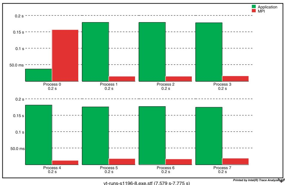
**Fig. 10** **a** Communication versus computation traces for all processors for Type-3 parallel SA. **b** Ratio of communication to computation for each processor for Type-3 parallel SA
