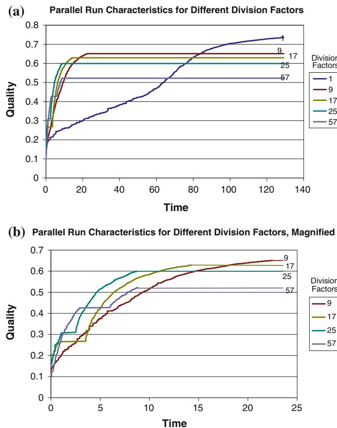
**Fig. 8** Quality versus runtime results for AMMC parallel SA (7 processors), with different values for  $M$
