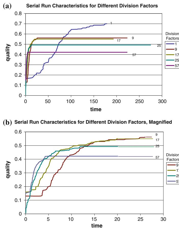
**Fig. 7** Quality versus runtime results for Serial SA, with different values for  $M$
