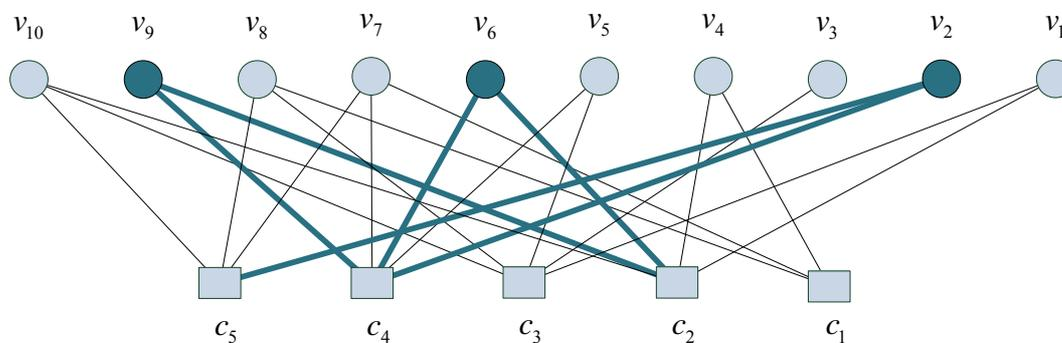
Figure 7: An example of a  $(3,2)$  trapping set  $T = \{v_2, v_6, v_9\}$
