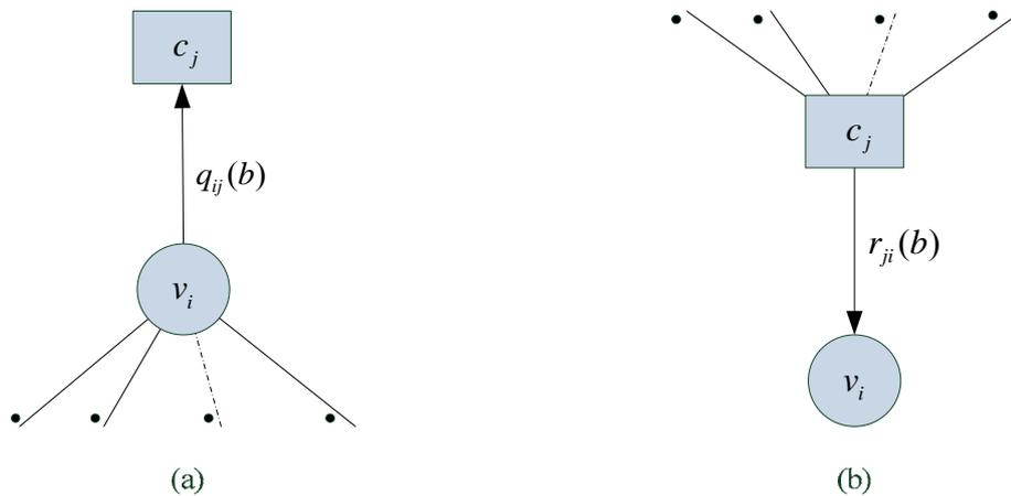
Figure 2: (a) Variable-to-check message, (b) Check-to-variable message
