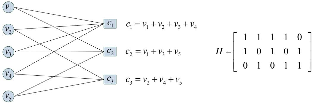
Figure 1: The two representations of LDPC codes: graph form and matrix form
