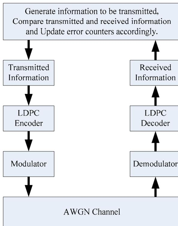
Figure 3: Block diagram of a conventional LDPC performance evaluation simulator
