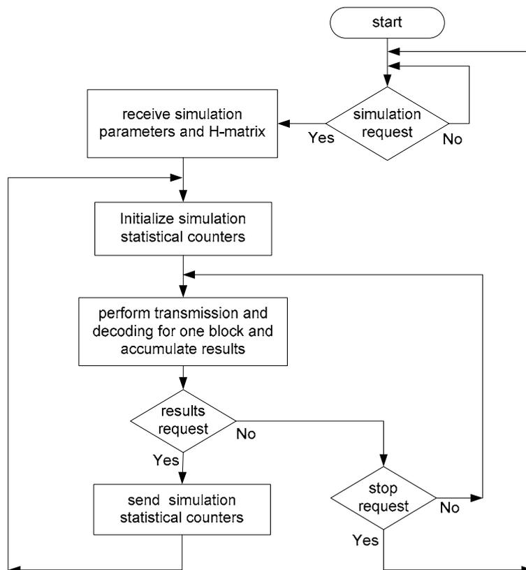
Figure 6: Processing node protocol
