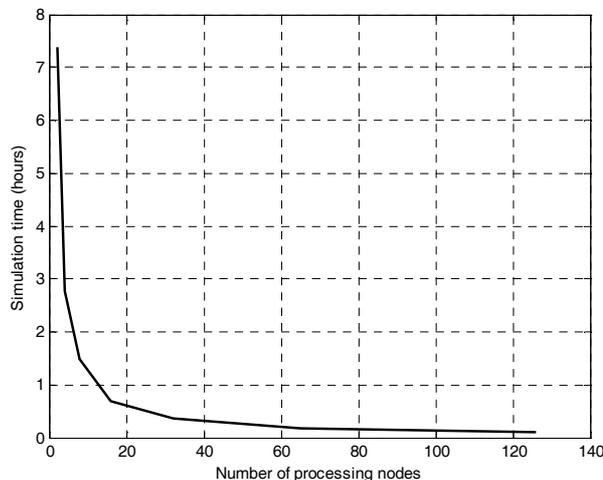
Figure 11: Simulation time vs number of processing nodes
