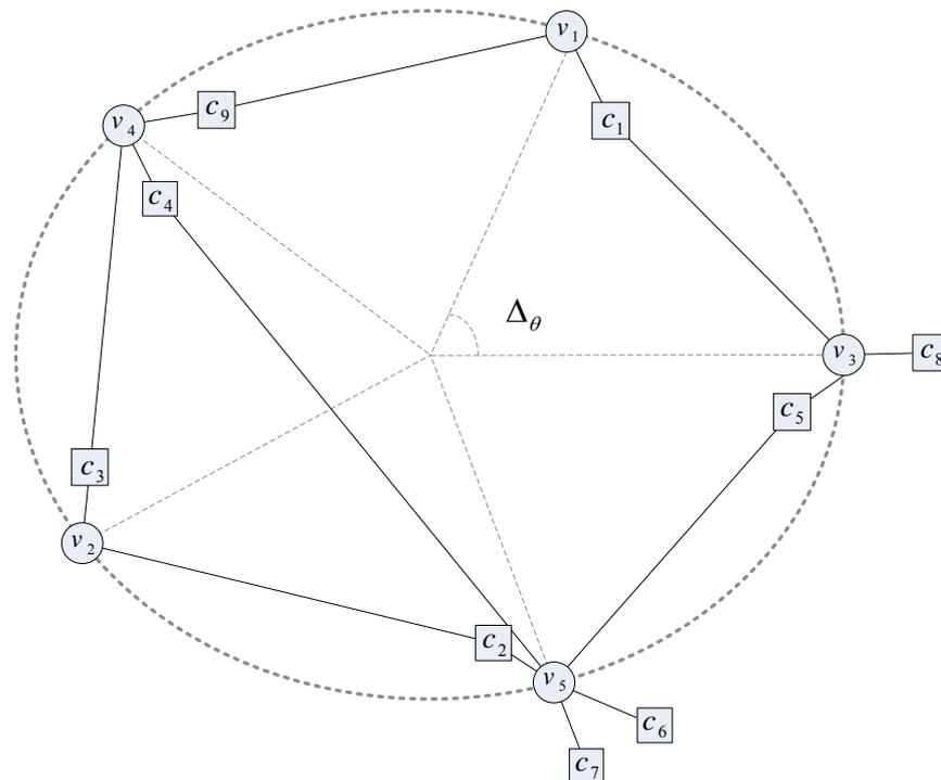
Figure 8: An example of variable and check nodes placement
