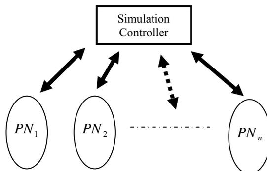
Figure 4: Components of the proposed parallel LDPC simulation platform
