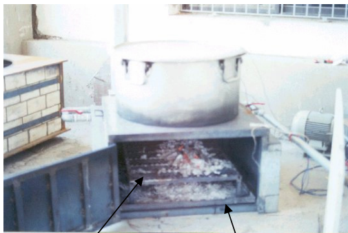
Figure 6.c MS-2 stove during test operation Grate Bottom Plate
