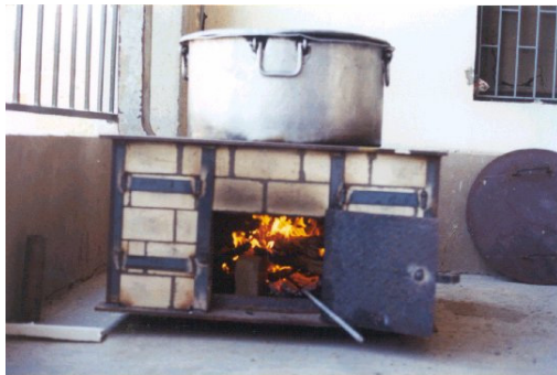
Figure 6.a FBS stove during test operation
