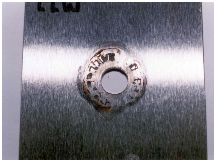
Figure 5. Close-up view of crevice attack on 410 SS in LLW
