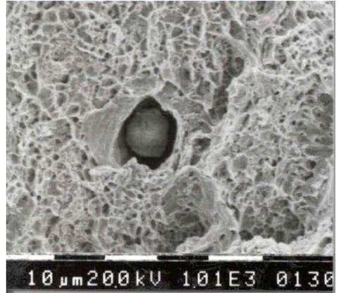
Fig. 12 A microalloy precipitate in ductile matrix.
