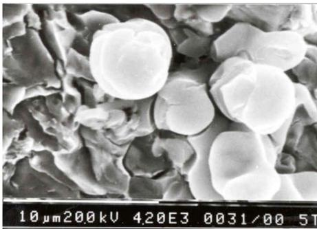
Fig. 13 An Aggregate of inclusions as HIC site.
