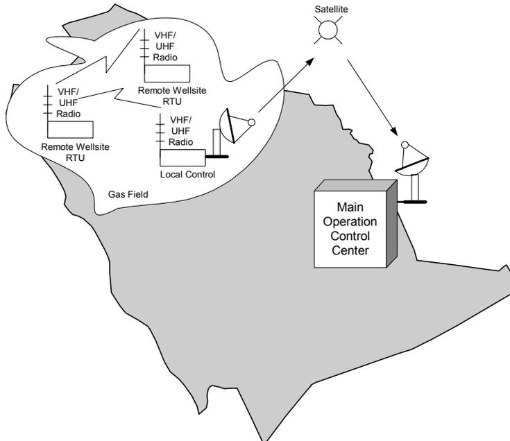
FIGURE III: SCADA COMMUNICATIONS EXAMPLE
