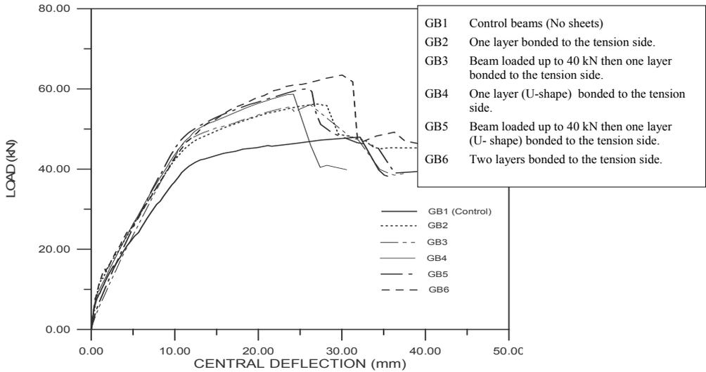
Figure 2: Load-deflection relationship for the second series of specimens
