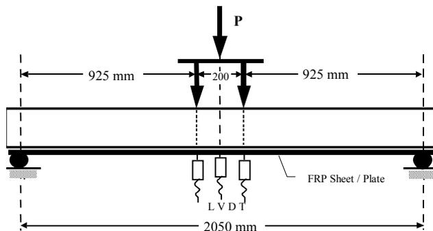
Figure 1: The test setup for flexural specimens
