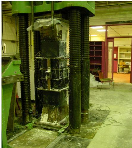
Figure 5. Test setup for column specimen of second series specimens.
