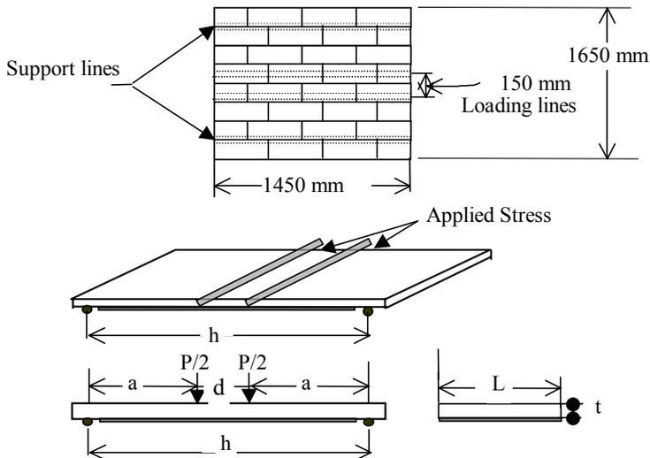
Figure 10: The test setup and dimensions of the out-of-plane block wall specimen.
