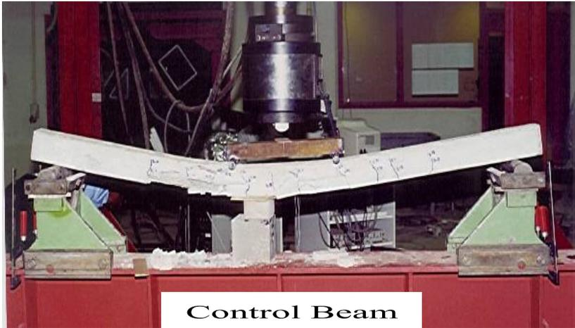
Fig. 5 The control beam after flexure test.
