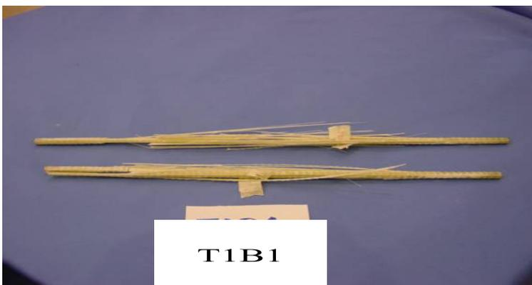
Fig. 7 The bars of T1B1 beam after tension test.
