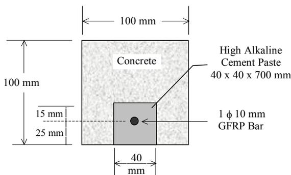
(b) Beam cross-section (Section A-A)
