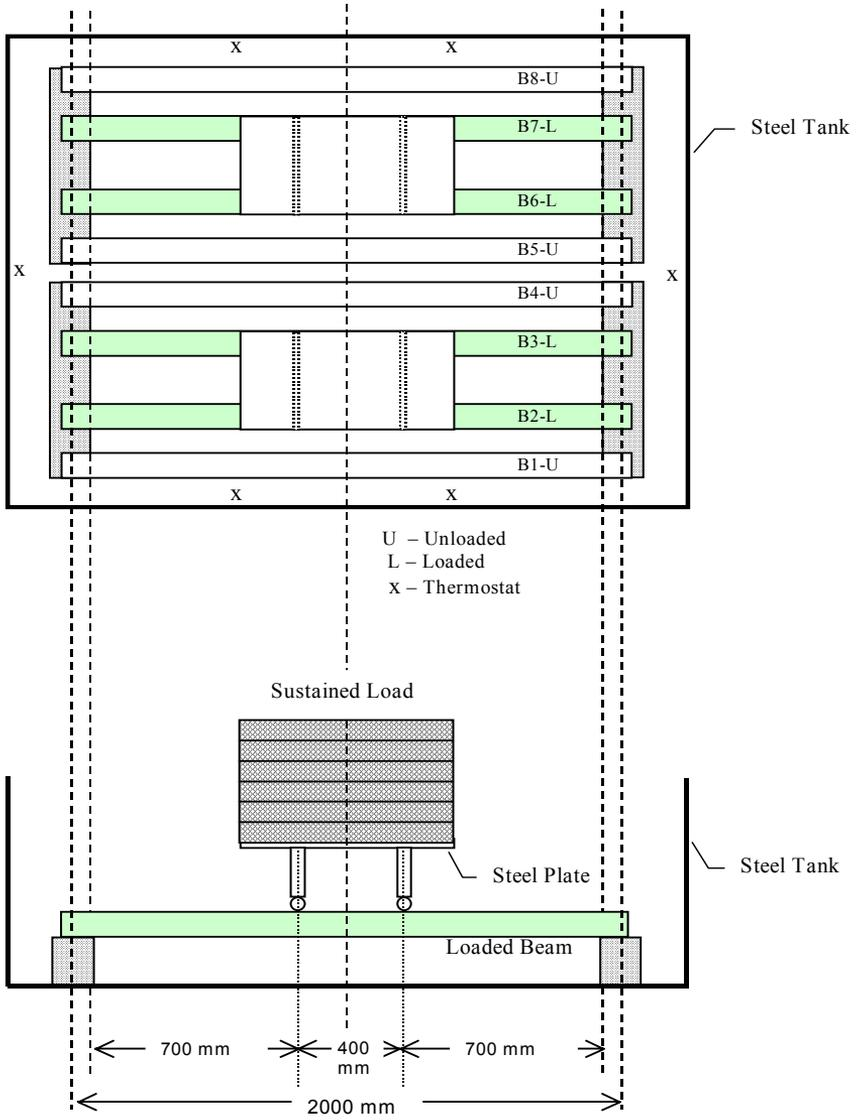
Fig. 2 Arrangement of specimens in each tank.
