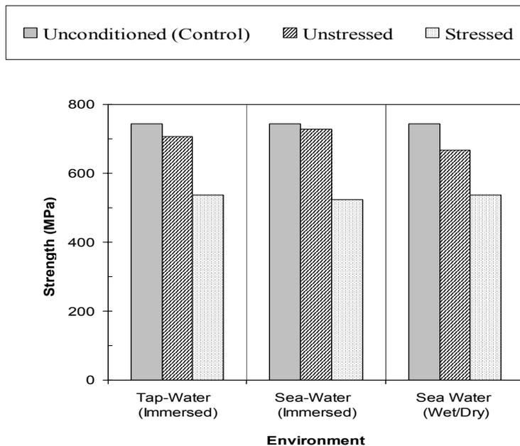
Fig. 3 The average tensile strength variation for all GFRP bars tested after 4 months under all exposure conditions at 40°C.
