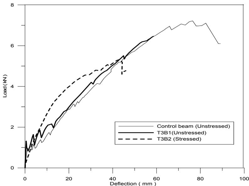
Fig. 4 The load-deflection relationships for beams tested after 4 months of exposure in tank 3 (wet/dry cycles of sea water exposure)
