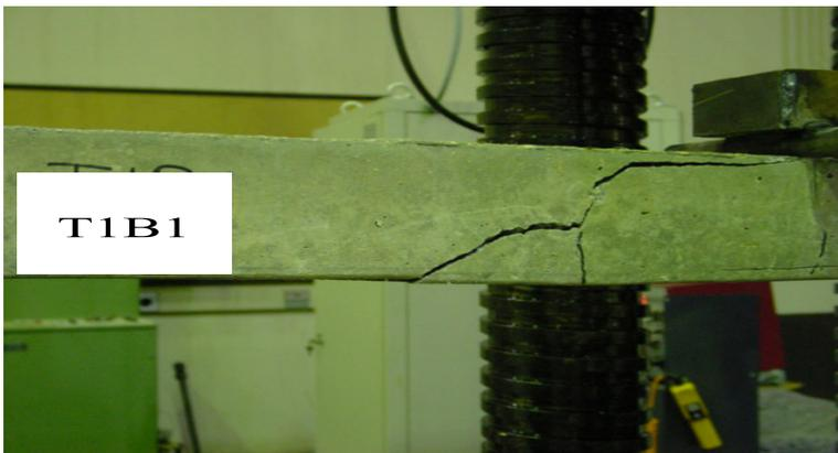
Fig. 6 The T1B1 beam after flexure test
