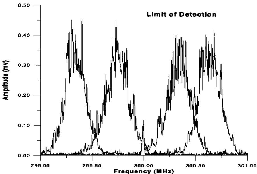
Figure: 2 Typical Doppler shifted signals indicating the resolution limit of our system.
