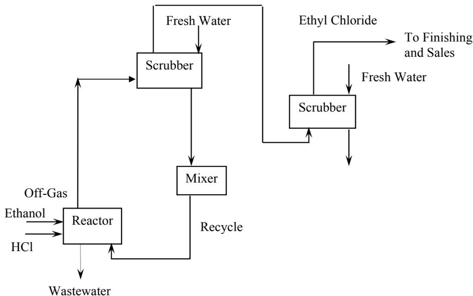
Figure 2: Ethyl Chloride Process
