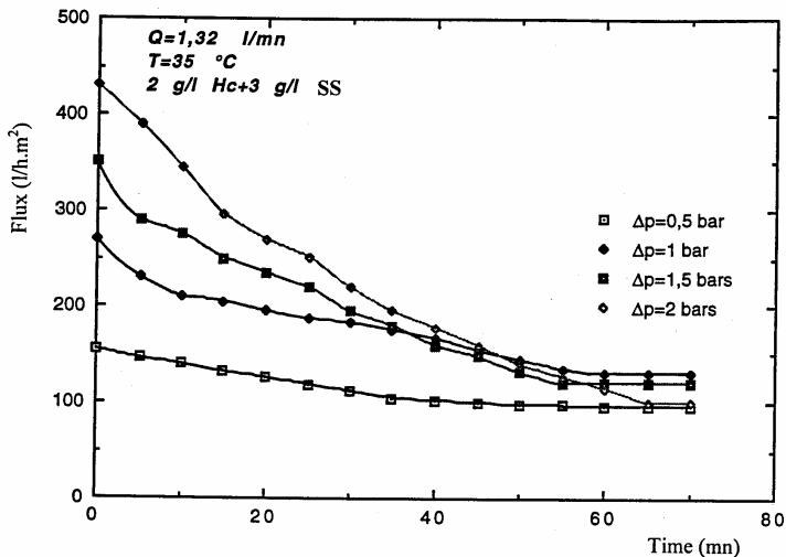
Figure 6: Flux against time at various pressures in presence of helical baffles
