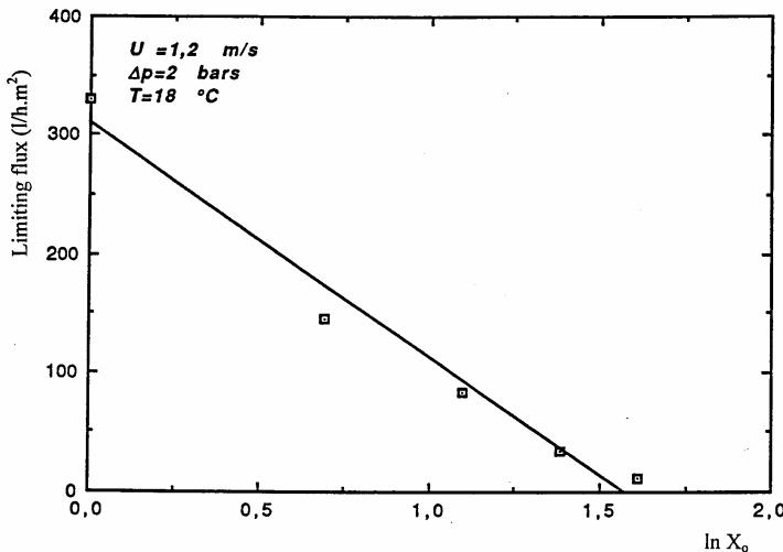
Figure 7: Limiting flux against  $\ln x_o$
