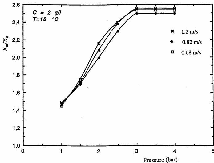
Figure 10:  $x_m/x_0$  against driving pressure
