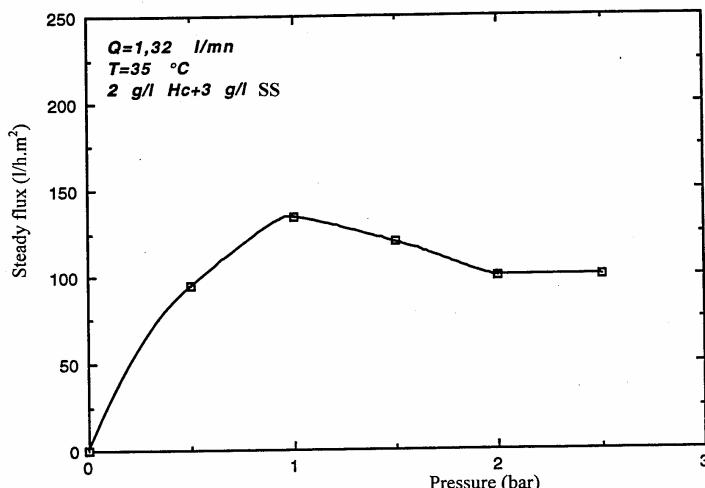
Figure 12: Steady flux against pressure with baffle
