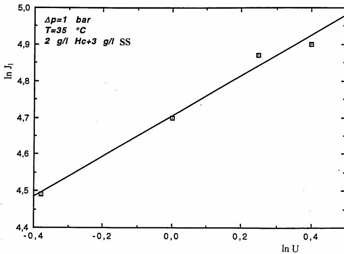
Figure 9:  $\ln J_l$  against  $\ln u$
