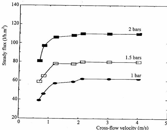
Figure 8: Steady flux against cross-flow velocity, 2 g/l HC, 18 °C
