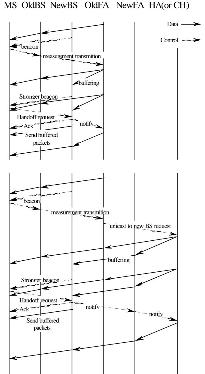
Fig. 2: Forced Hand off Algorithm
