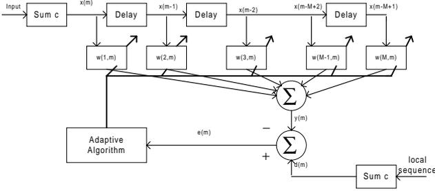
Fig. 1. Schematic of an Adaptive Filter for the proposed Code Acquisition System
