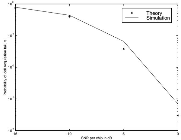
Fig. 2. Theoretical and Simulation results for Probability of Cell Acquisition Failure against  $SNR_c$  for a system using spreading sequence of 127 chips.
