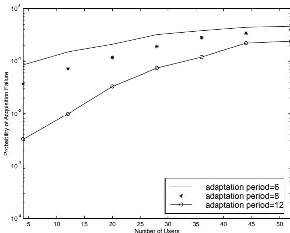
Fig. 3. Probability of Acquisition Failure as a function of Number of users for different values of Adaptation periods with  $SNR_c$  of  $-5$  dB
