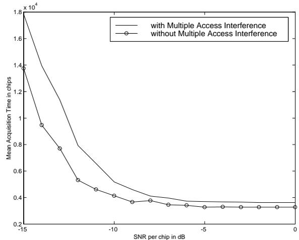
Fig. 4. Mean Time to Acquisition in chip periods against  $SNR_c$  (signal-to-noise-ratio per chip in dB) in the presence of MAI (4 users )
