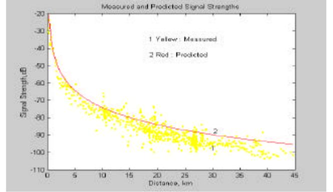
Figure 6 Actual and Predicted Signal Strengths Using Hata
