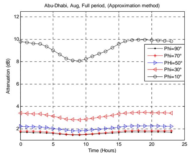
Fig. 14. Hourly averaging of gases attenuation at different elevation angles
