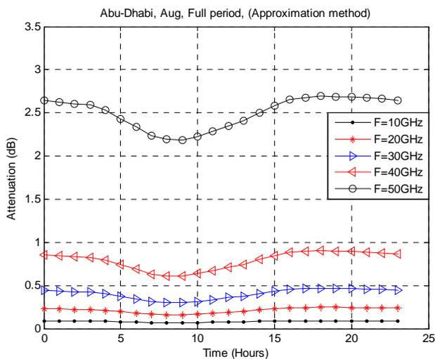
Fig. 13. Hourly averaging of gases attenuation at different frequencies
