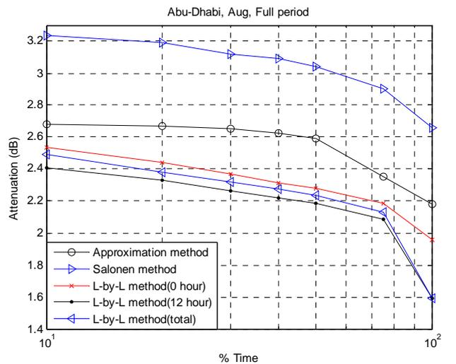
Fig. 8. Cumulative distribution of gases attenuation in Abu-Dhabi
