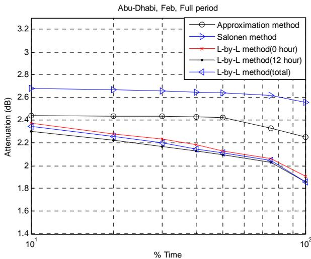
Fig. 7. Cumulative distribution of gases attenuation in Abu-Dhabi
