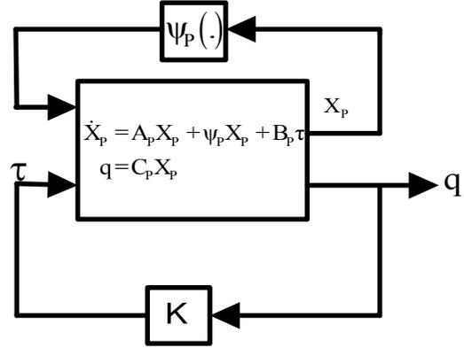
Fig. 2. Small gain theorem implementation.
