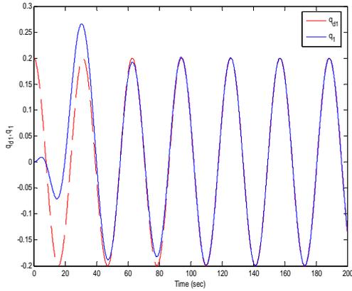
Fig. 3. Internal Model principle based attitude tracking  $q_{d1}(t)$ ,  $q_1(t)$
