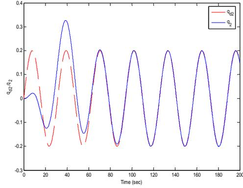
Fig. 5. Internal Model principle based attitude tracking  $q_{d2}(t)$ ,  $q_2(t)$
