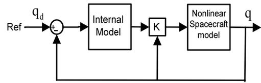
Fig. 1. Internal Model principle based spacecraft attitude control
