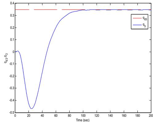
Fig. 7. Internal Model principle based attitude tracking  $q_{d3}(t)$ ,  $q_3(t)$
