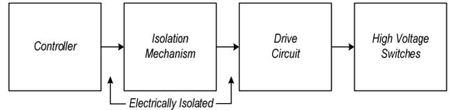
Figure 4: An illustration of solid state device based pulser topology
