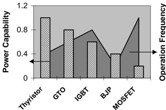
Figure 1: Features available with different solid-state devices.
