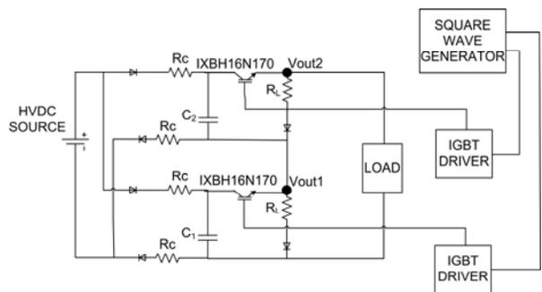
Figure 5: A schematic of a cascade type square-wave pulse generator showing two stages.
