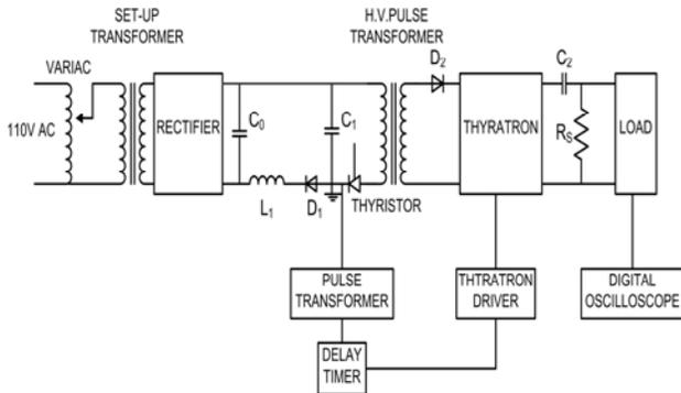
Figure 3: A schematic of a high repetition thyatron based pulsed power supply.
