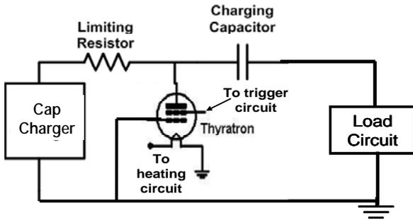
Figure 2: A schematic of a thyatron-based pulsed power supply.
