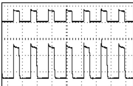
Figure 6: Train of square pulses generated by a four-stage cascaded pulser (Figure 5). Upper waveform, at the output terminal of the first stage, and the lower waveform is at the last (fourth) stage terminal. Scale: x-axis: 500V per division and y-axis: 500  $\mu$ s.
