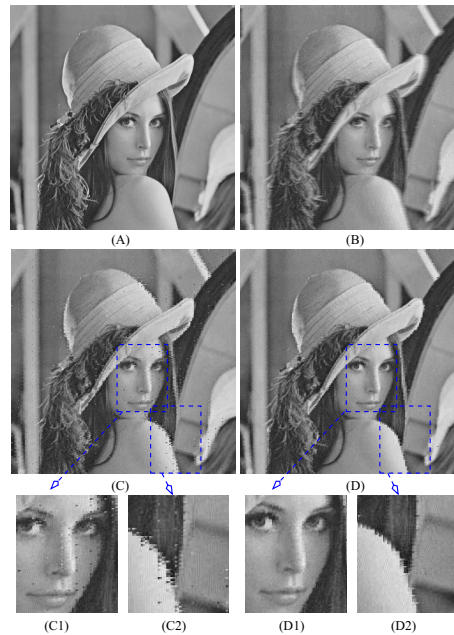
Fig. 4. Simulation results for Lena image. (A.) is the 256 \times 256 original image. (B.) represents the results for 1-bit quantizer using fixed \eta raster scan, Figures (C.) and (D.) represent the 1-bit quantizer using adaptive \eta Morton(Z) scan without and with smooth boundary, respectively.
