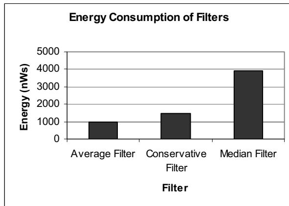
Fig 4: Energy consumption requirements for filters
