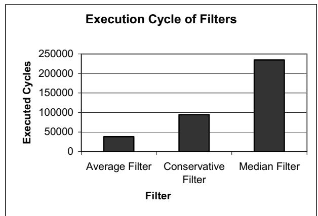
Fig 6: Execution cycles taken by Filters
