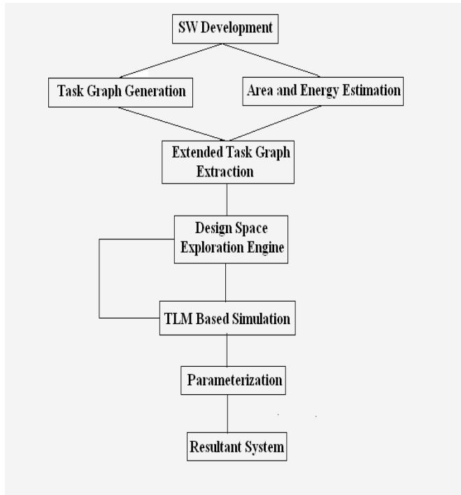
**Fig. 2 HW/SW Codesign Flow**
