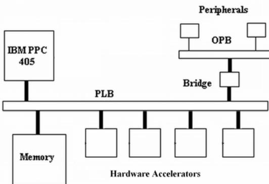
**Fig 1: Target Platform Built using IBM TLM**
