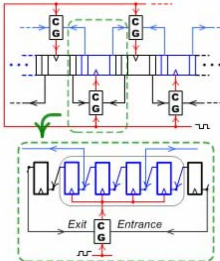
Fig. 5. Hot Block architecture for ring counters. – The ring counter is partitioned into  $b$  blocks of size  $s$  ( $s$  is 4 in this figure). – The complexity of the clock gators remains unchanged with varying block sizes.
