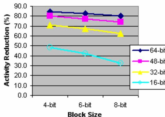
Fig. 7. The activity reductions for ring counters of different width and block sizes as compared to the conventional ring counter
