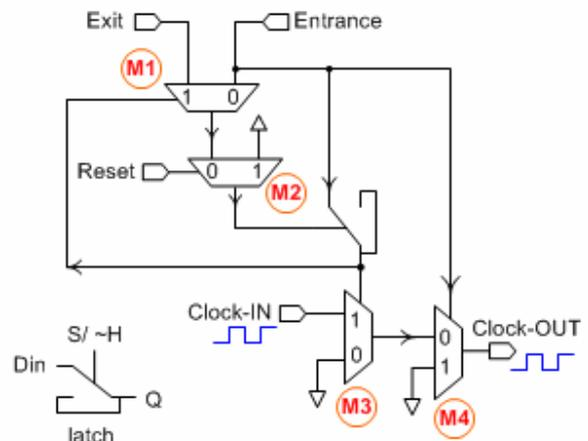
Fig. 6. The Hot Block clock gator used in the Hot Block architecture (Fig. 5) – Whatever the block size is, there are only two inputs (*Entrance* and *Exit*) coming from other blocks.
