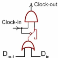
Fig. 2. The single bit clock gator logic. -  $D_{in}$  and  $D_{out}$  are flip-flop's input and output respectively.
