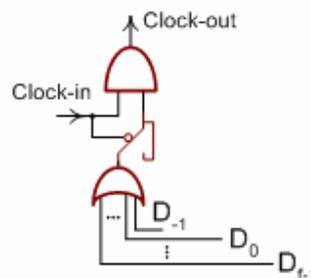
Fig. 4. The multiple bit clock gator logic. - For a block with  $f$  flip-flops, the OR gate has  $f+1$  inputs. -  $D_{-1}$  is connected to the leftmost bit of the righthand block.
