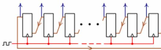
Fig. 1. The conventional synchronous ring counter [5]
