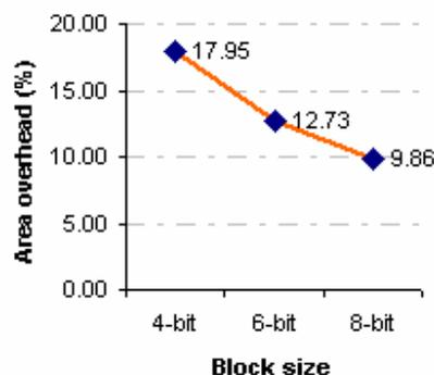
Fig. 9. The area overhead for different block sizes – as expected smaller blocks have larger area overheads
