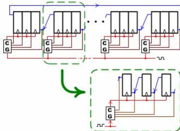
Fig. 3. Using a single clock gator for multiple (3 here) flip-flops
