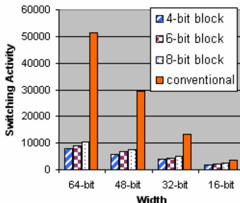
Fig. 8. Switching activities of different ring counters – *Hot Block* ring counters raise noticeably fewer signal transitions. – Best results are obtained in *Hot Block* ring counters with blocks of size 4.
