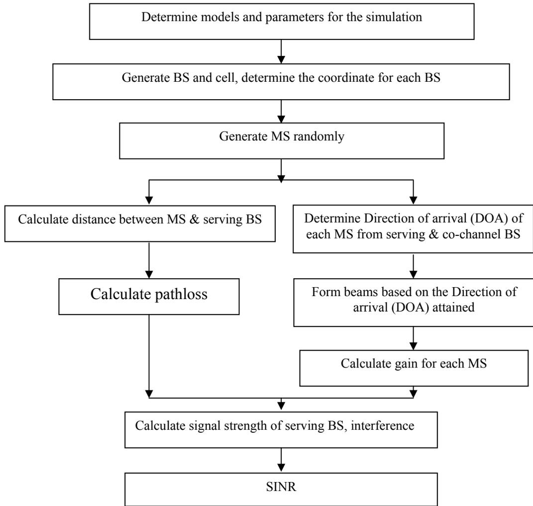
**Figure 3:** Flowchart of simulation cycle
