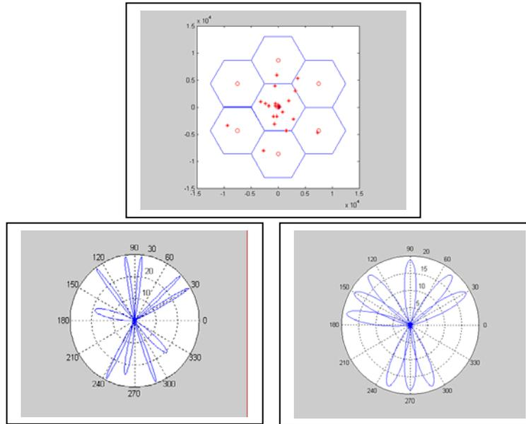
Figure 4: Cell topology (7 BSs, 20MSs), beam pattern at BS 1 by adaptive and switched beam antenna respectively.
