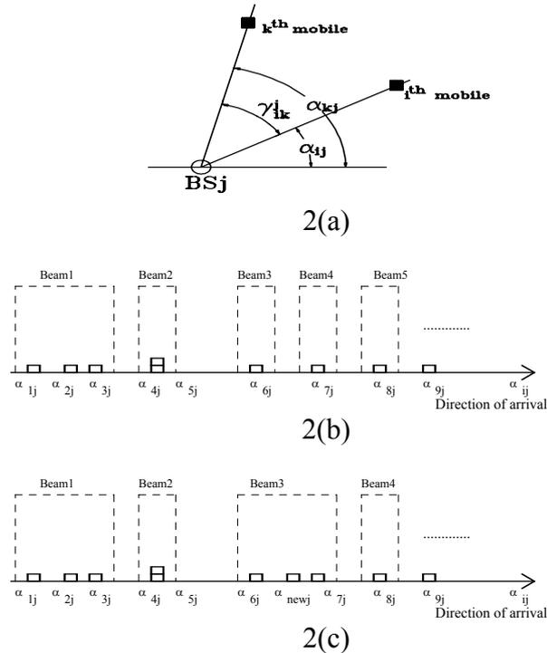
**Figure 2:** (a) Actual beam formation algorithm parameters, (b) Examples of beam formation and (c) Beam reformation to accommodate a new call
