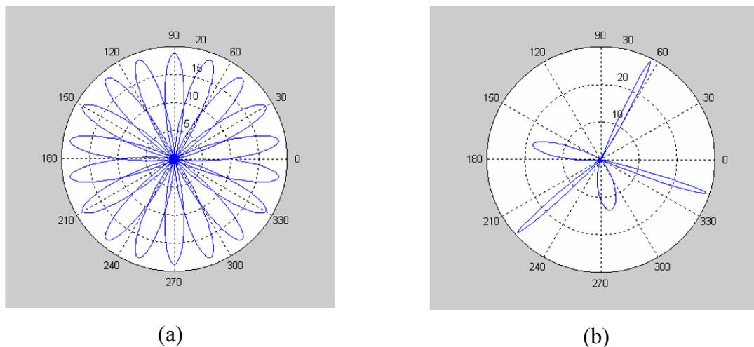
**Figure 1:** Typical antenna pattern for (a) switched beam and (b) adaptive beam
