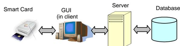
Figure 6. Main components of the smart card system
