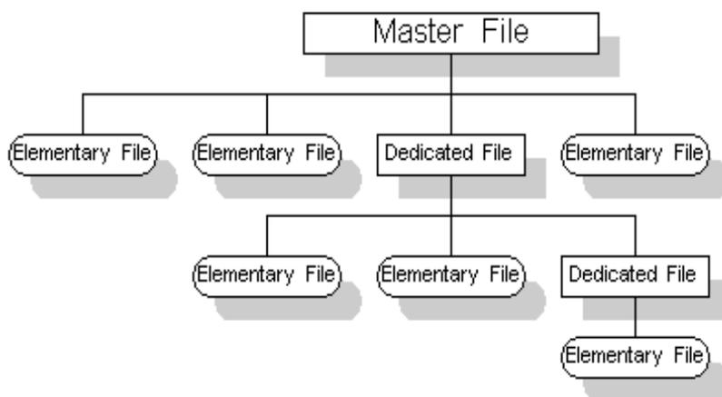
Figure 1. Logical file structure of smart card
