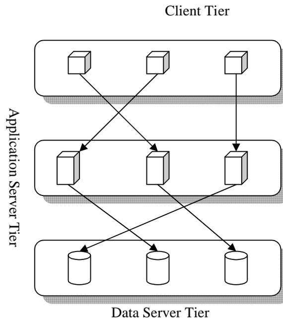
Figure 5. Three Tier architecture
