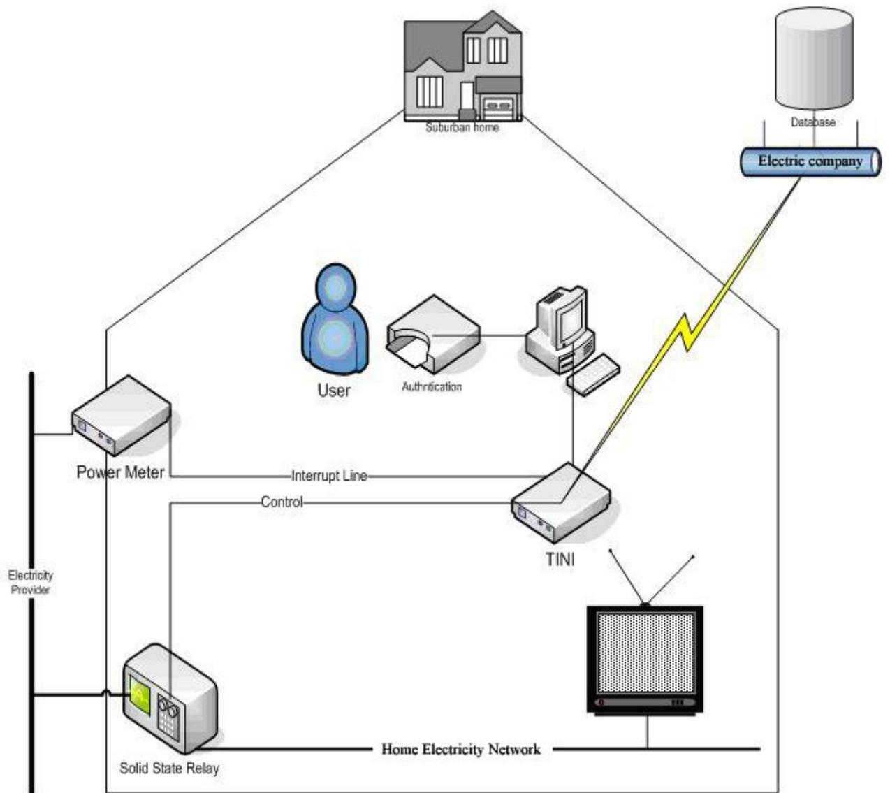
Figure 2 Prepaid Electricity System Design
