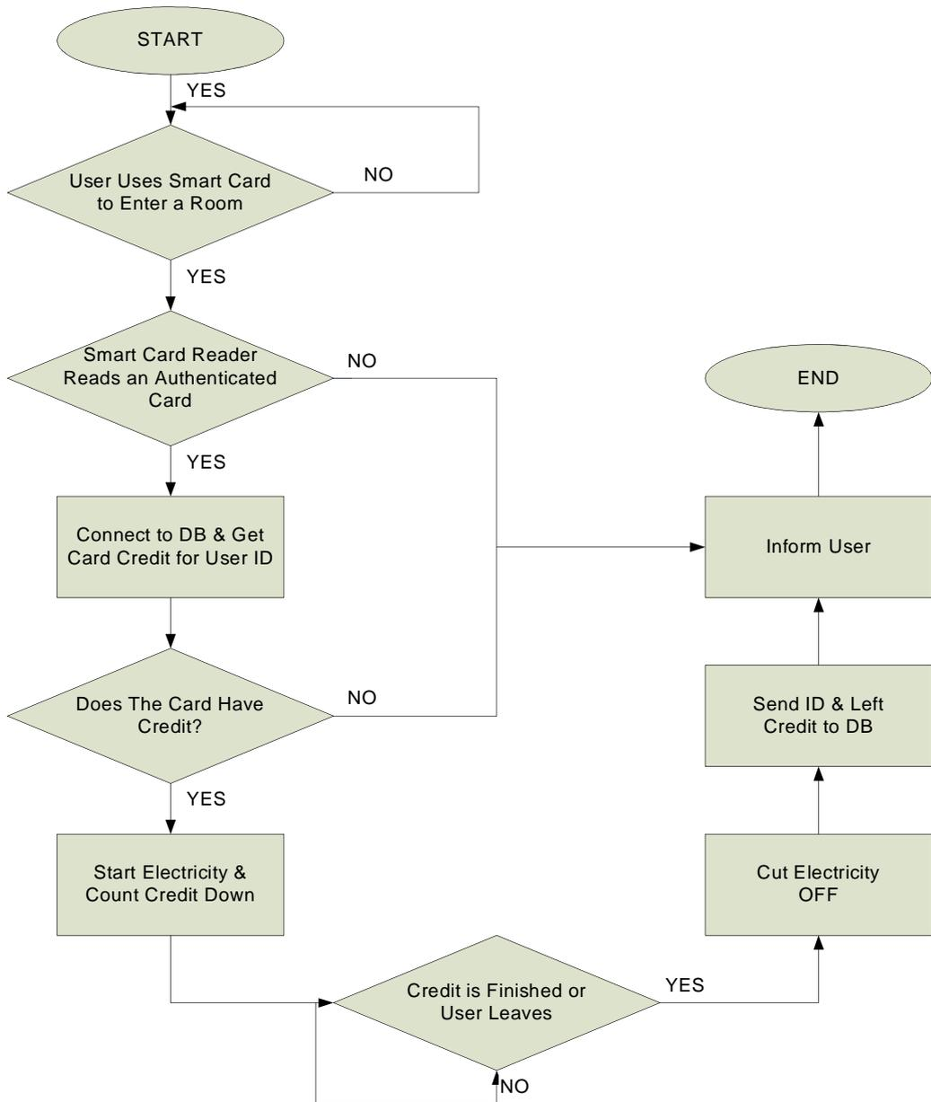
Figure 3. Flow Chart for Prepaid Electricity
