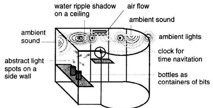
Figure 1: ambientROOM schematic diagram
