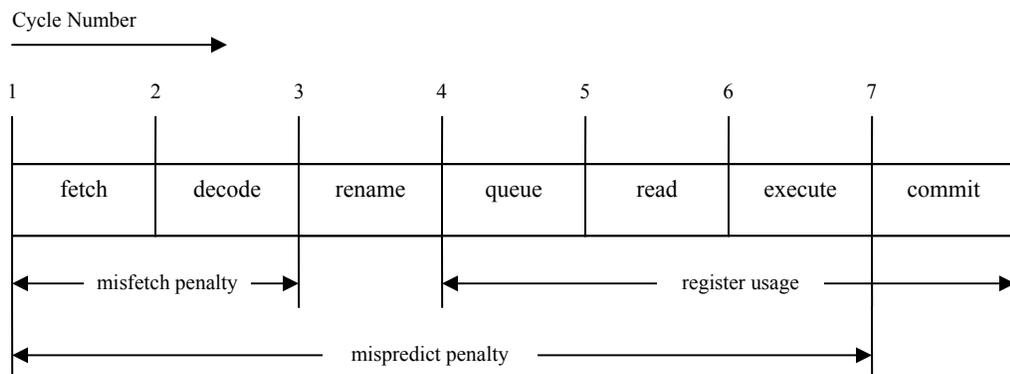
Figure 4. Superscalar Pipeline
