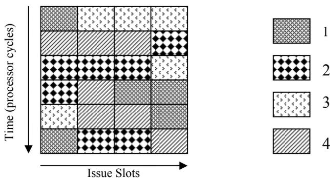
(b) Issue Slot Partitioning of 4 threads in an SMT Processor
