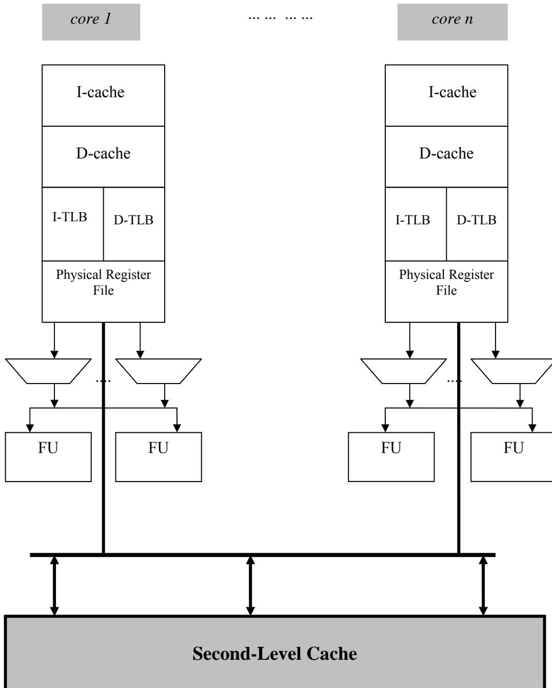
Figure 3. General View of the Proposed Microarchitecture
