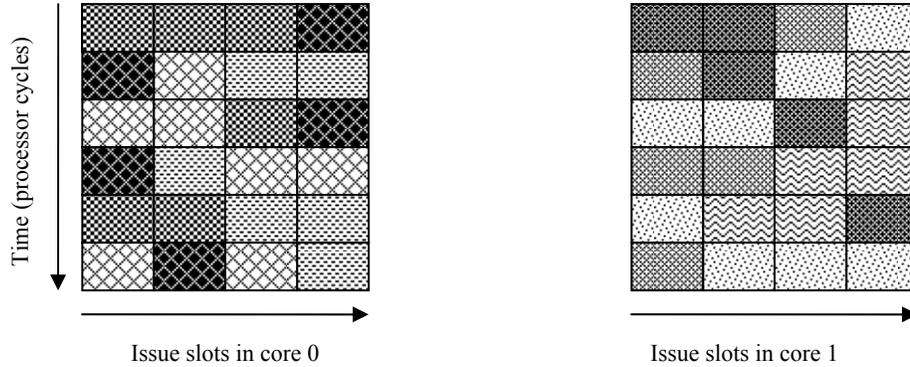
Figure 2. Issue Slot Partitioning in Chip Multi-Threading (CMT)
