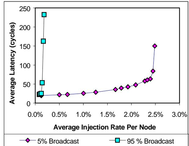
Figure 12: Injection Rate in a 16x8x8 Mesh with a different mix of unicast and broadcast messages
