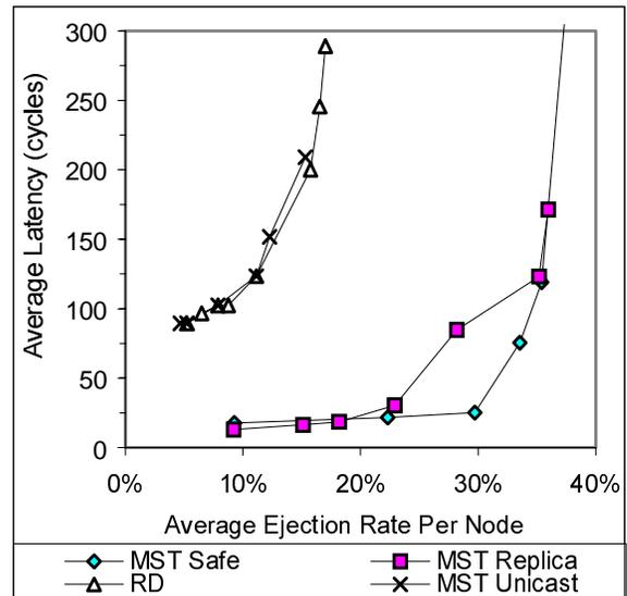
Figure 8 : Latency and Ejection Rate in an 8x8x8 Mesh
