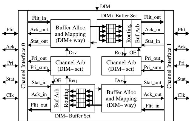
Figure 2: Internal Structure of a Router
