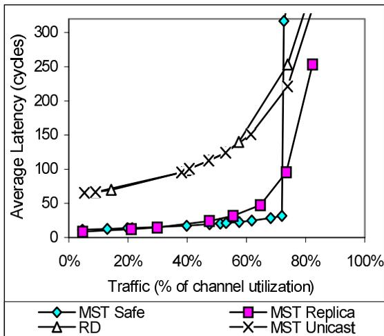
Figure 11: Latency and Traffic in 9D Hypercube
