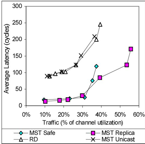
Figure 9: Latency and Traffic in an 8x8x8 Mesh
