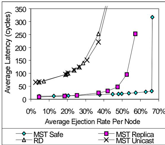
Figure 10: Latency and Ejection Rate in a 9D Hypercube
