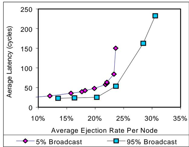
Figure 13: Ejection Rate in a 16x8x8 Mesh with a different mix of unicast and broadcast messages
