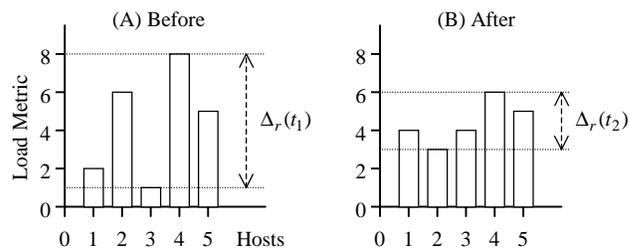
Figure 4: Loads of 5 hosts before and after balancing
