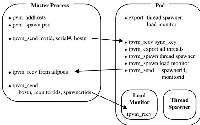
Figure 3: Creating a pod and setting the load monitor and thread spawner.
