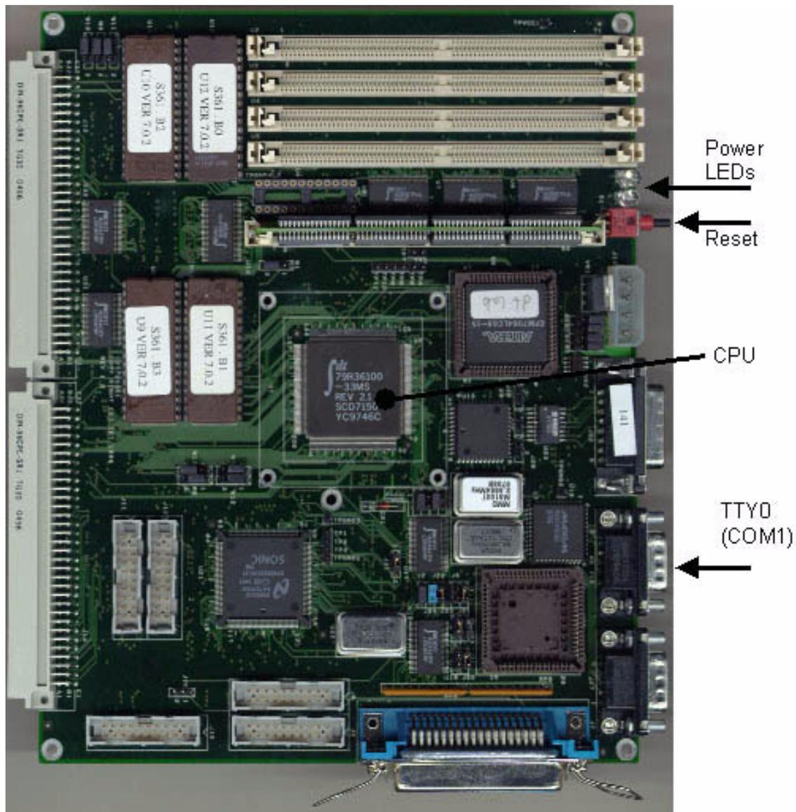
FIGURE 1 The lab board (not including the I/O expansion card).
