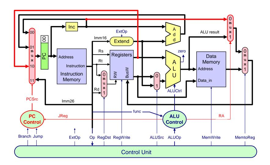
The necessary changes to the datapath and control are shown in red.
