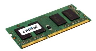
♦ Example: 64-bit data bus using 4 × 16-bit DRAM chips
