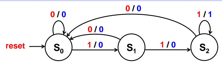
Input test sequence: reset then x = 0, 1, 0, 1, 1, 0, 1, 1, 1, 1
