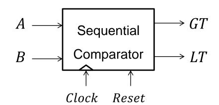
Compare  $A_0$  with  $B_0$ ,  $A_1$  with  $B_1$ , etc. (Bit 0 is least significant bit)
