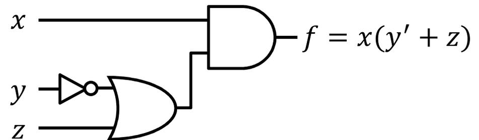
Truth Table and Logic Diagram describe the same function  $f$ . Truth table is unique, but logic expression and logic diagram are not. This gives flexibility in implementing logic functions.
