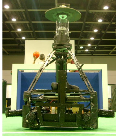
Figure 3. Tribot, omni-directional drive and camera
