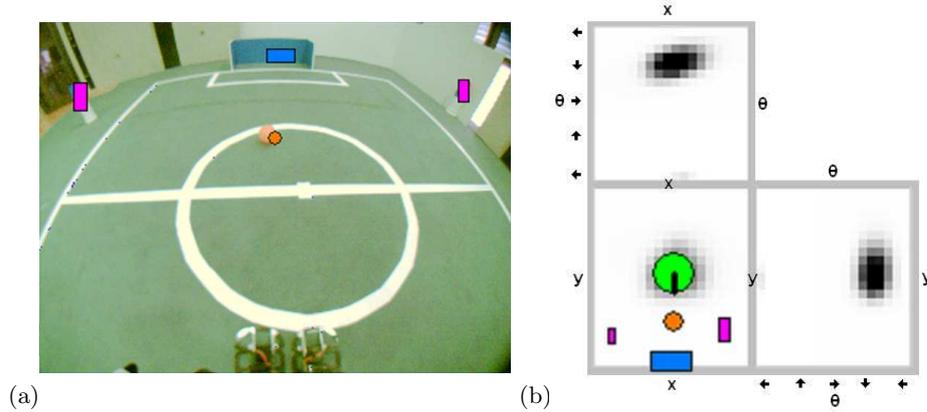
**Fig. 4.** (a) Image captured from Toni’s perspective while it was walking. Detected objects: goal (blue horizontal rectangle), ball (orange circle), and pole (magenta vertical rectangle); (b) Three 2D projections of the 3D grid representing the probability distribution of robot poses  $(x, y, \theta)$ . The green circle is drawn at the estimated robot location  $(x, y)$ . The black line represents its estimated orientation  $\theta$ . The detected objects are drawn relative to the robot.
