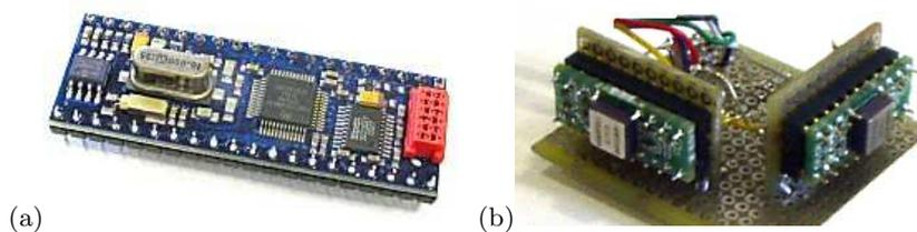
**Fig. 2.** Electronics: (a) ChipS12 microcontroller board featuring HCS12C32; (b) Attitude sensor consisting of a dual-axis accelerometer and two gyroscopes.
