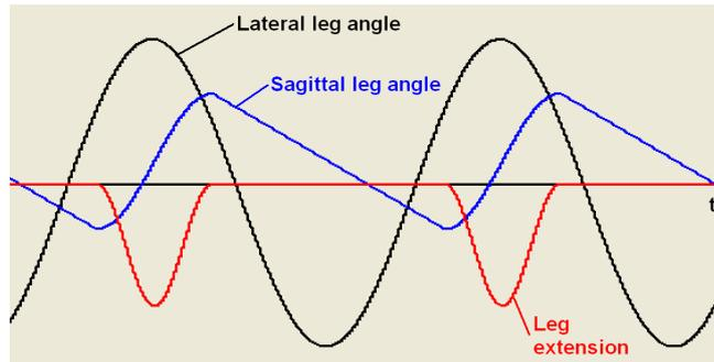
**Fig. 5.** Dynamic walking. Leg angles and leg extension of a leg while walking forward with small steps. The other leg moves in the same way, with a phase offset of  $\pi$ .
