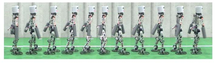
Fig. 6. Image sequence extracted from video of forward walking robot (every second frame).
