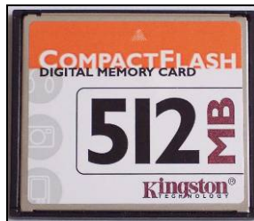
Figure 6. Typical Compact Flash Memory Card
