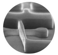
Intel 30nm Tri-gate Transistor
