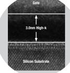
Future High-k Dielectric for Reduced Gate Leakage
