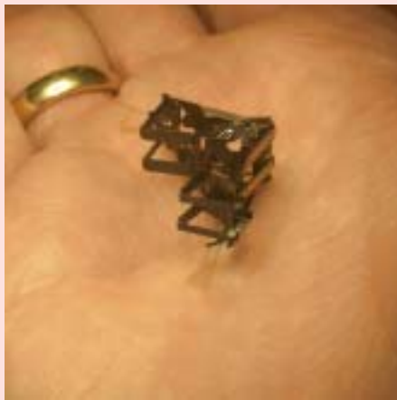
Flying insect; micromachined C fiber; 100mg weight, 30 mm wing span
