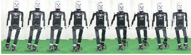
Fig. 4. Sequence of every other frame extracted from video showing an entire step of the walking robot (frontal view).
