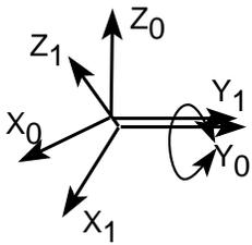
Fig 2.7: R1 rotates around its Y axis.
