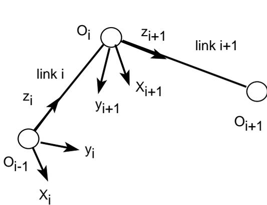
Fig 2.19: Two links with a revolute joint
