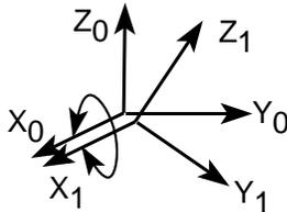
Fig 2.8: R1 rotates around its X axis.
