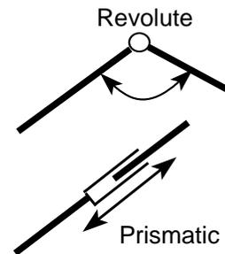
Fig 2.13: A revolute joint and a prismatic joint.
