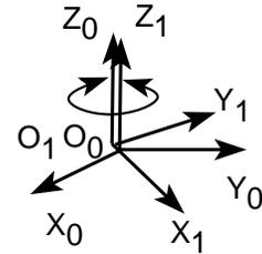
Fig 2.6: R1 rotates around its Z axis.
