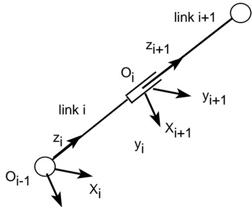
Fig 2.20: Two links with a prismatic joint
