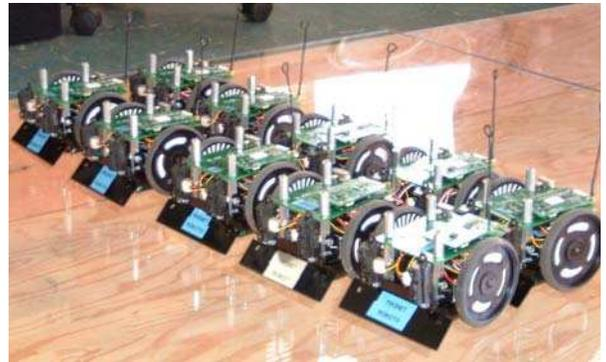
Fig. 1. Ten Mica2-based robots for the MAS-net project.
