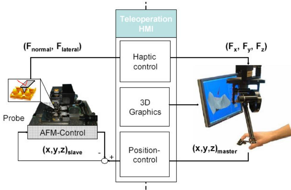
Figure 4: Human Machine Interface setup (Vogl, 2004).
