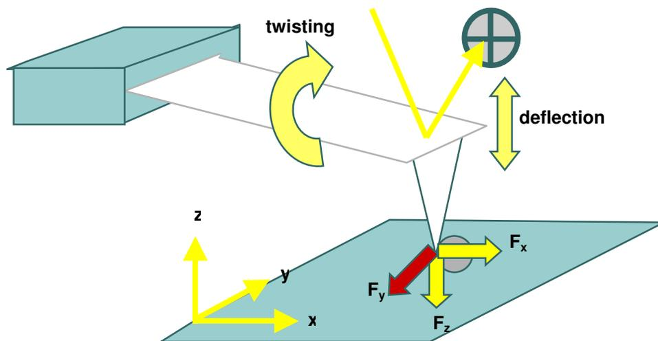
Figure 3: Force breakdown for cantilever during surface interaction.
