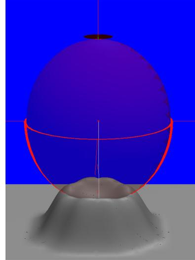
Figure 2: a) Force distance curve during approach to and retraction from a flat surface (Sitti, et al; 2003). b) Neck forming during retraction.
