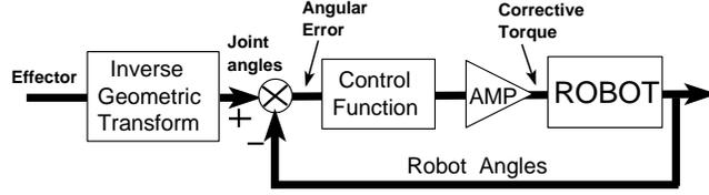
a - Motion coordination using the geometric model
