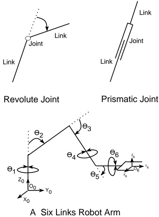
Figure 1.1: General schematic of a robot arm
