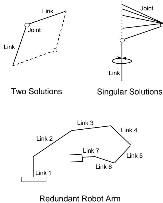
Figure 1.2: Multiple solutions, singular solution, and redundant arms
