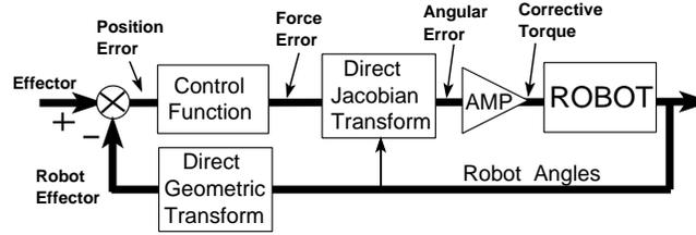
c - Motion coordination using the virtual work concept
