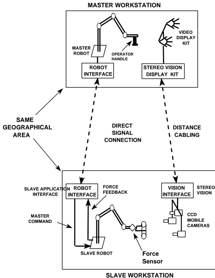
Figure 1.6: Telerobotics system: master and slave station are in one area
